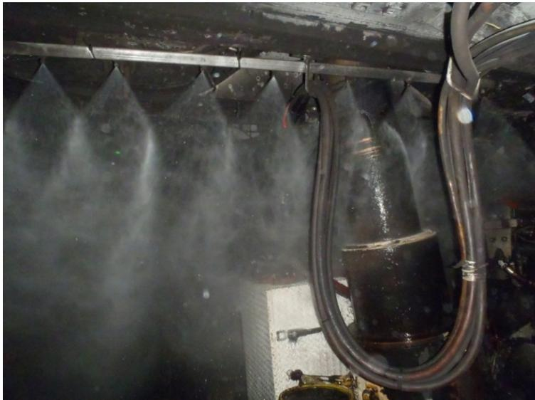
**Figure 9: Face partition sprays installed on a shield canopy**
