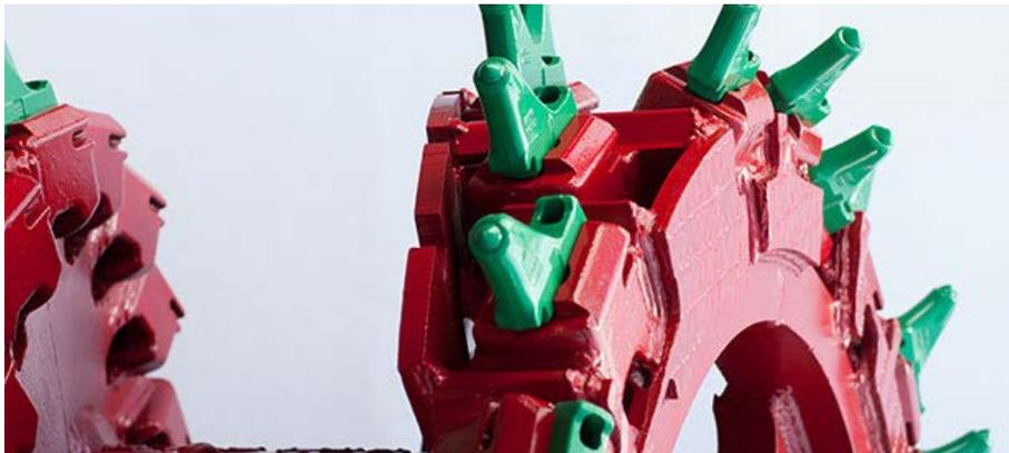
Figure 19: Shearer drum fitted with Radial picks
