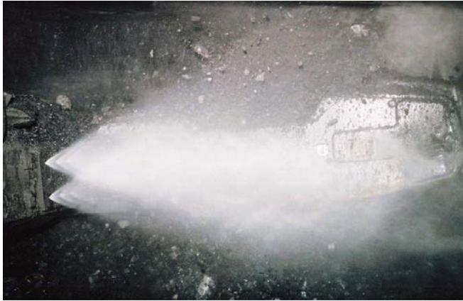
**Figure 22: Side sprays on Tailgate ranging arm**
