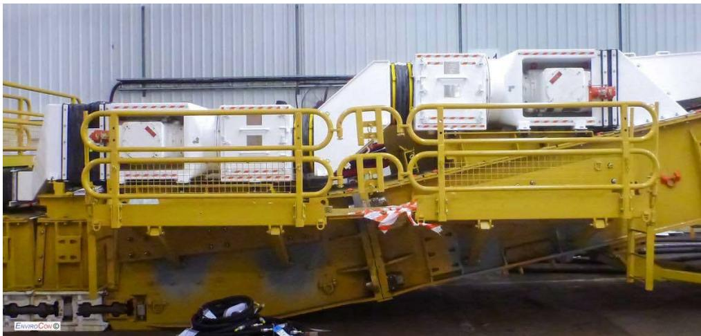
Figure 2: Scrubber fan system mounted on BSL
