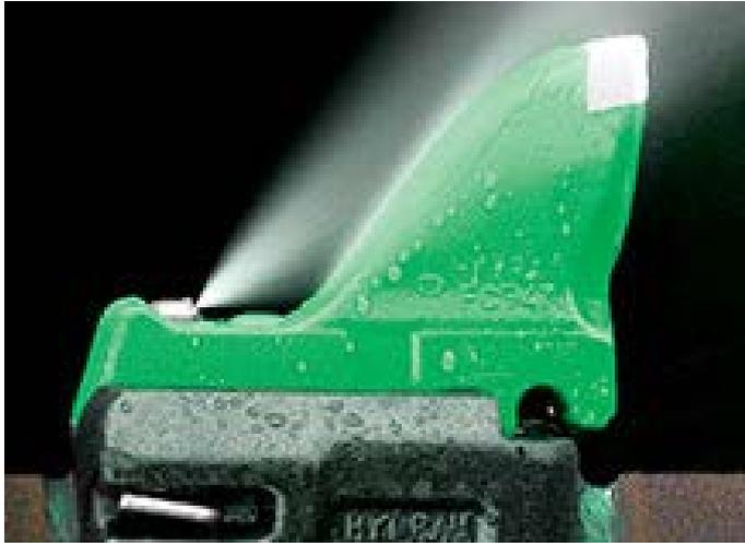
**Figure 14: Back flushing pick spray**
