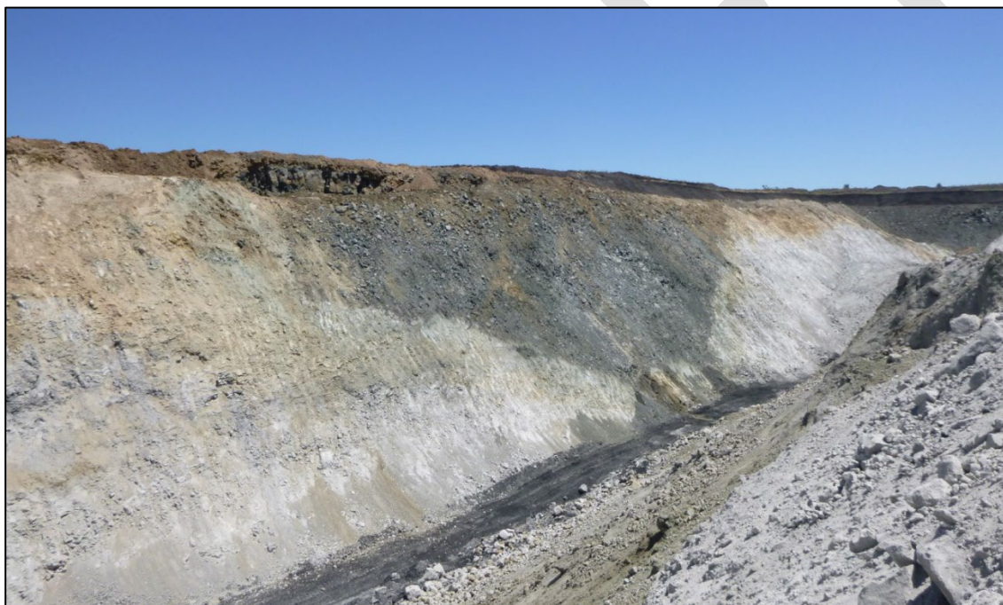
Figure 5: Example of variable geological conditions with hard igneous basalt overlying soft sedimentary formations
