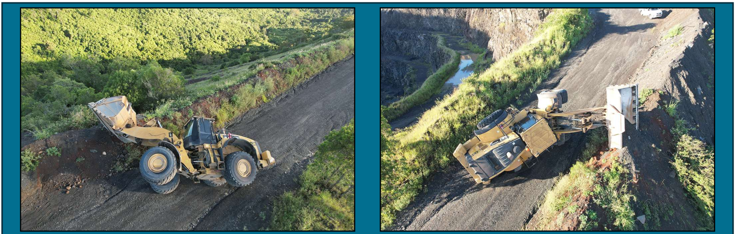
Figures 1 & 2 – Photos showing the rolled front-end loader
