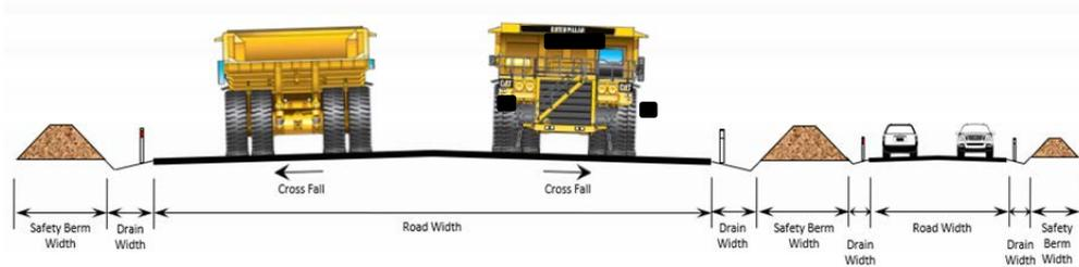
Where road width cannot be achieved an assessment of risk shall be undertaken to determine controls that manage the hazard to an acceptable level of risk (e.g. specifying give way requirements, speed restrictions, installation of narrow road signage highlighting the road width hazard etc.).
