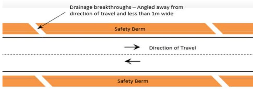
**Figure 5. Drainage breakthroughs in roadside safety berms**
