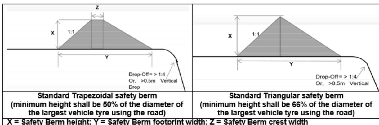
**Figure 6. Design requirements for standard Trapezoidal and Triangular safety berms**
