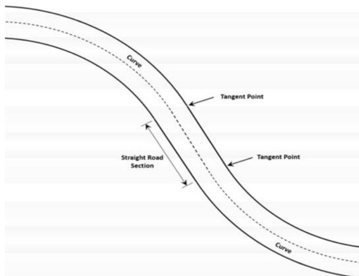
**Figure 2. Horizontal reverse curve**
