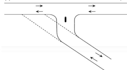
Figure 3. 'Y' intersection treatment example
