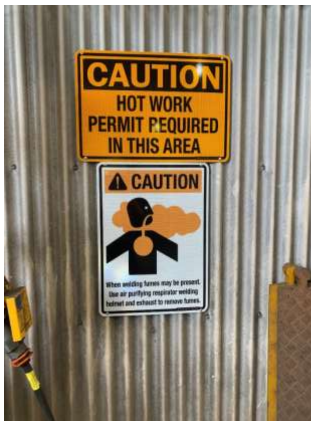
Figure A2: Clear signage on the hazards of welding in workshop where welding is conducted
