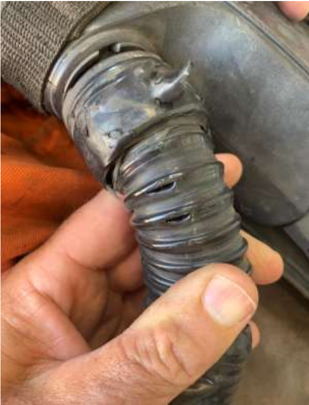
Figure A5: Compromised and poorly maintained PAPR
