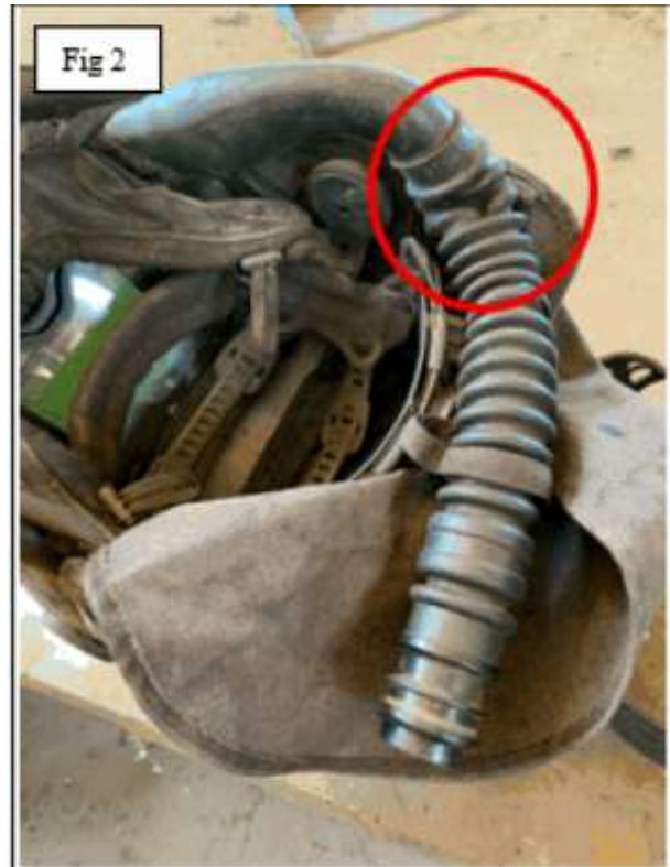
Figure A6: Compromised and poorly maintained PAPR
