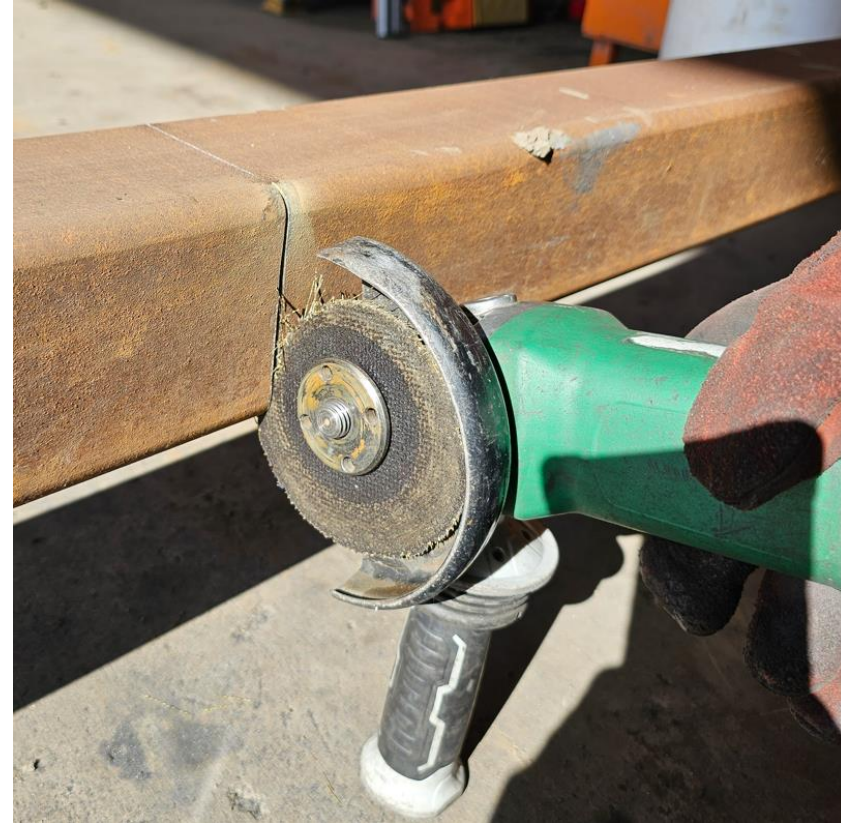
Re-enactment photo showing point at which grinder grabbed and kicked back
