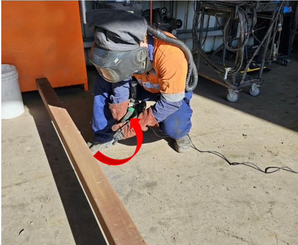
Re-enactment photo showing direction of movement by the grinder after kickback
