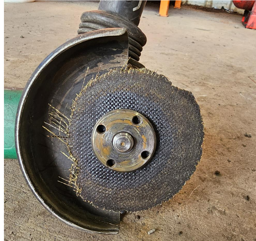
Photo showing condition of the disc after incident
