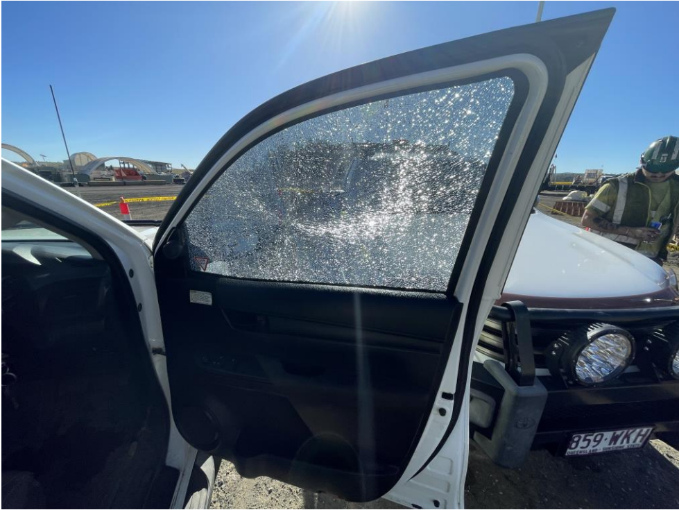
Light vehicle struck by concrete shattering passenger side window.
