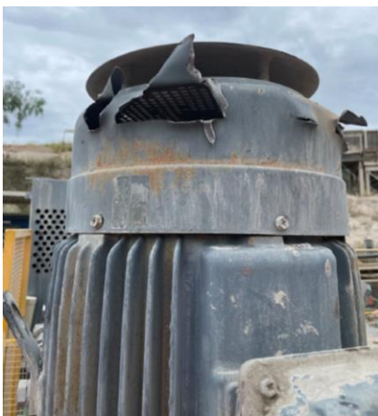
Photos showing fan fragment ejection damage
