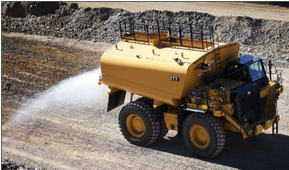
Photo 28: Water truck to mitigate roadway dust
