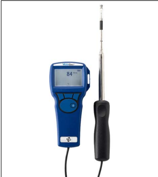
Photo 2: Hot Wire Anemometer
