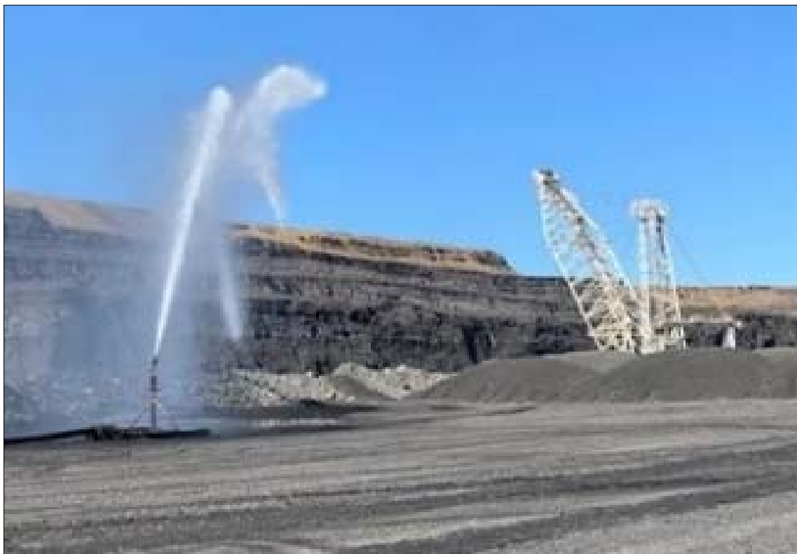
Photo 15: Wetting of blasted material
