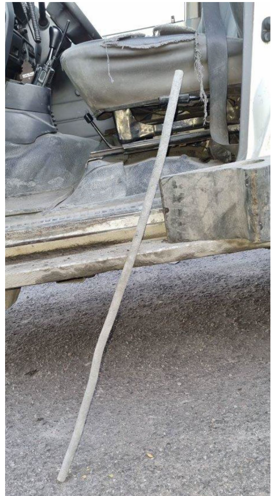
Figures 1 & 2 – Photo showing damage to LV floor and re-enactment showing likely rod position after floor was punctured
