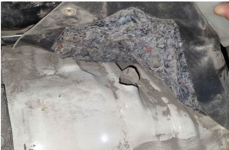
Figures 1 & 2 – Photo showing damage to LV floor and re-enactment showing likely rod position after floor was punctured
