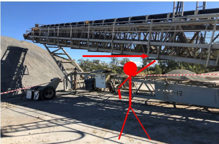
Photographs showing the radial stacker and the nip point
