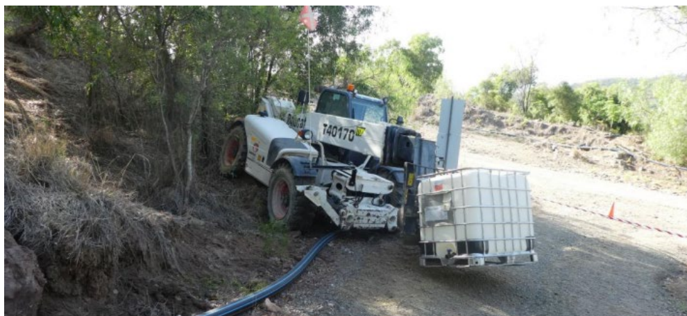
The telehandler came to a halt when it struck an earth embankment near an intersecting road
