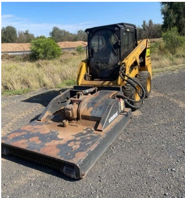
Figure 5-13 – Enclosed air-conditioned cab on roadside skid steer with slasher
