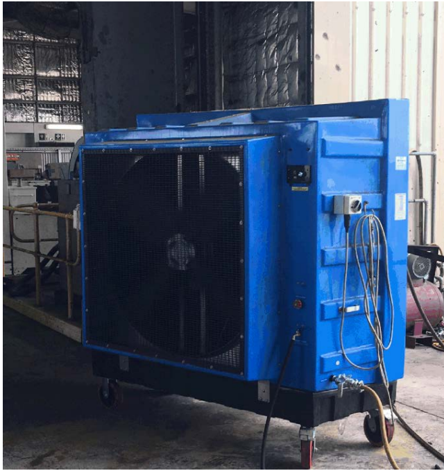
Figure 5-6 & 5-7 - Portable air-conditioned fan units provide cool air inside workshops
