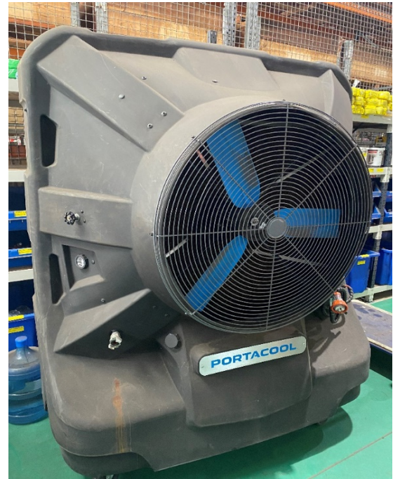
Figure 5-6 & 5-7 - Portable air-conditioned fan units provide cool air inside workshops
