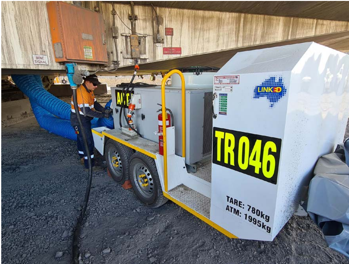
Figure 5-9 – Portable air-conditioning unit for dragline shutdowns
