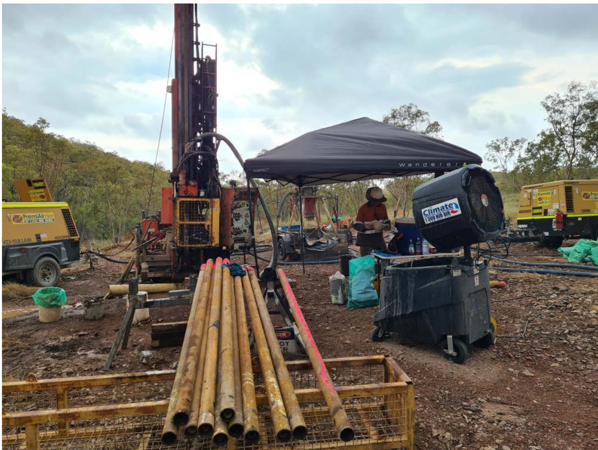
Figure 5-8 – Portable cooling fan directed at exploration drill operator position
